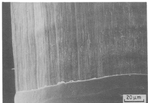
Figure 1 Immersion region of A: 10/65° C treated monofilament near meniscus.
